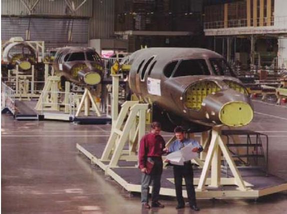
Figure 7 – Premier I fuselage shells with bulkheads
