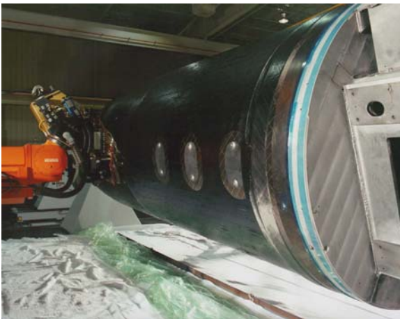
Figure 9 – The Viper placing carbon fibers on a fuselage
